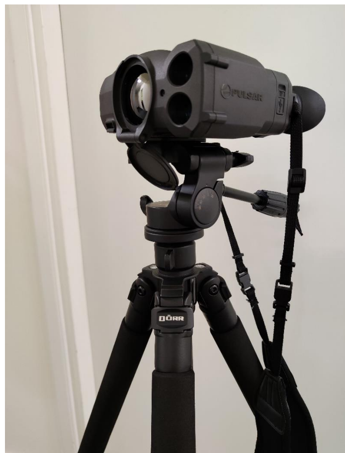
Figure 2-5 Thermal imaging camera Pulsar Accolade LRF XP50 on a tripod
