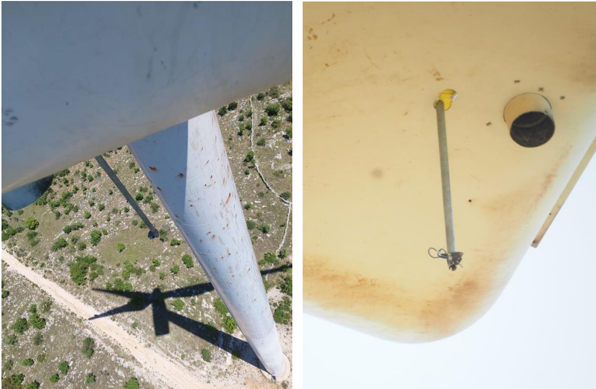
Figure 2-3 Microphone of ultrasound detector Elekon BATLOGGER WE X2 set at nacelle height (Photos: Vjetroelektrana Jelinak Ltd.)
