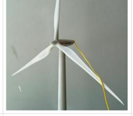
The emergency descent system line was displaced into the rotor sweep zone and became entangled on one of the blades.
