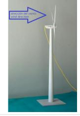
Turbine situation when the drill commenced: the nacelle was disorientated by 180°, with the wind blowing from the rear.
