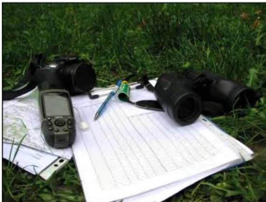
Figure 2 Ornithological fieldwork equipment: binoculars, a GPS device, a map of the area, camera and field forms (Photo: E. Patčev)
