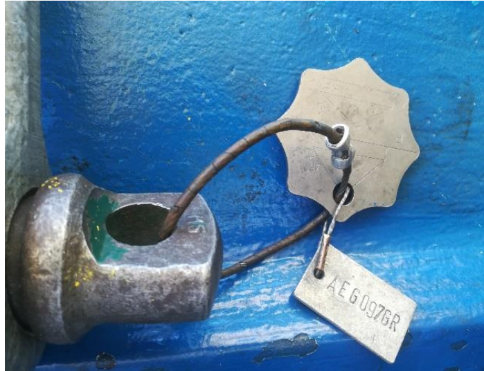
Detail of ring securing identification plate to shackle.
