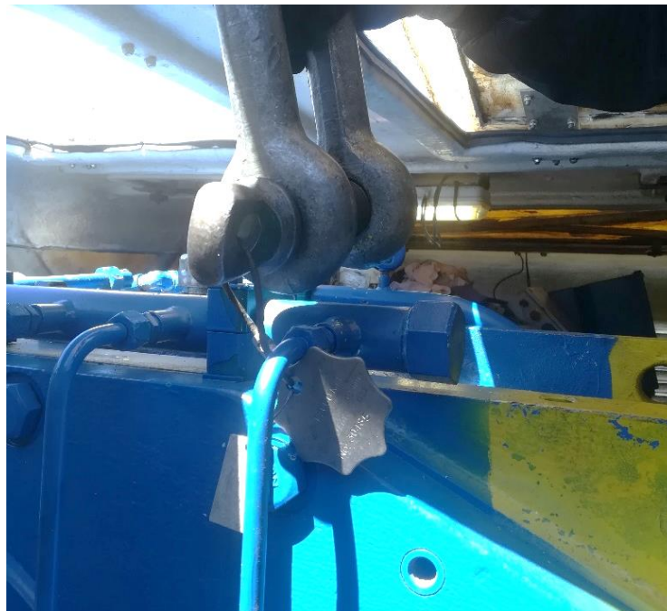
Shackle identification plate caught on one of the gearbox hoses.
